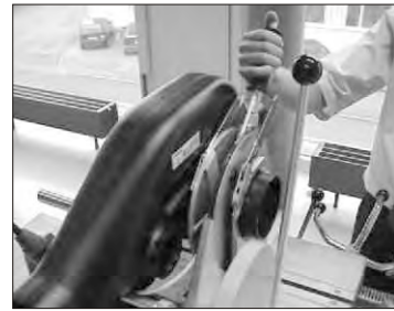
4. Grind the end port
