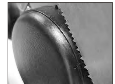
3、 Cut the end port according to required diameter
