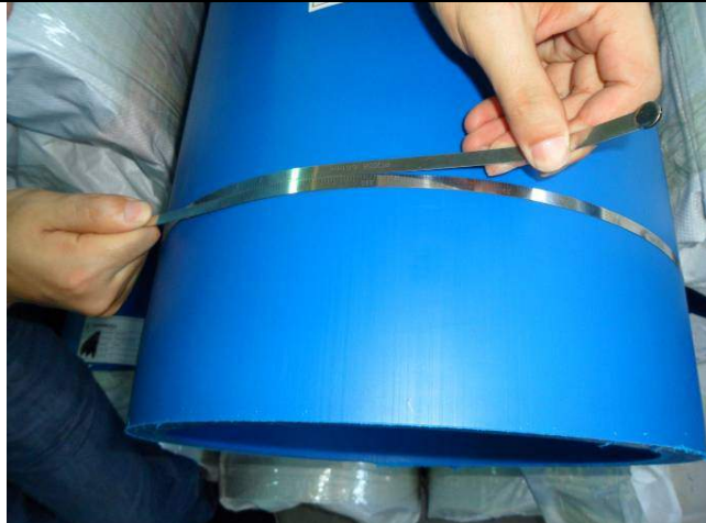
Mean outside diameter check of PE pipe
