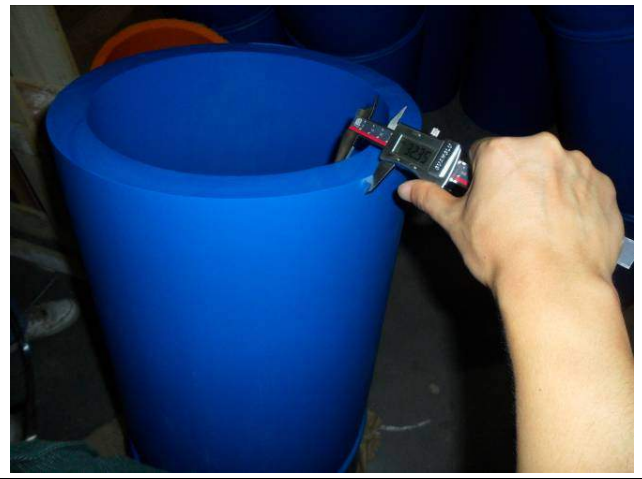
Wall thickness check of PE fitting
