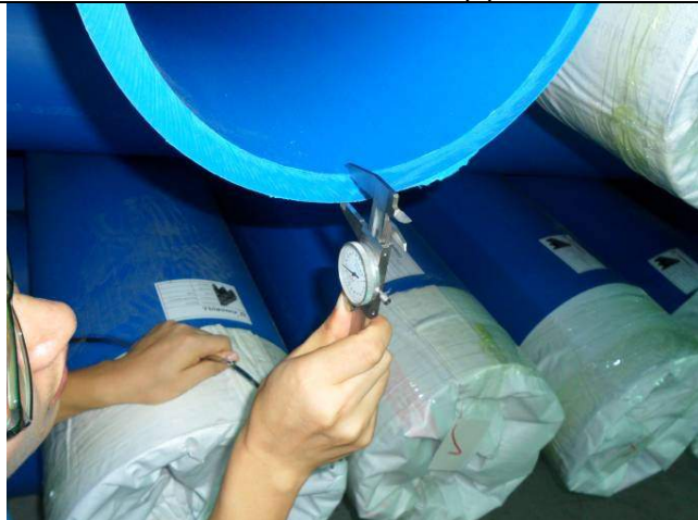
Wall thickness check of PE pipe
