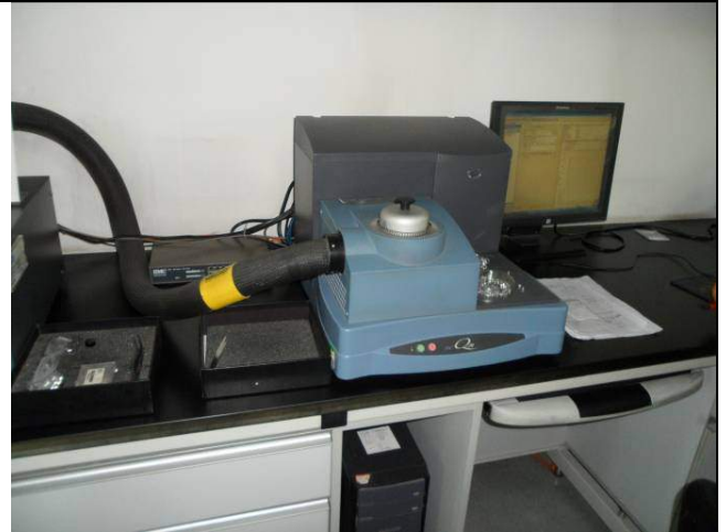
Oxidation induction time(OIT) 200°C test
