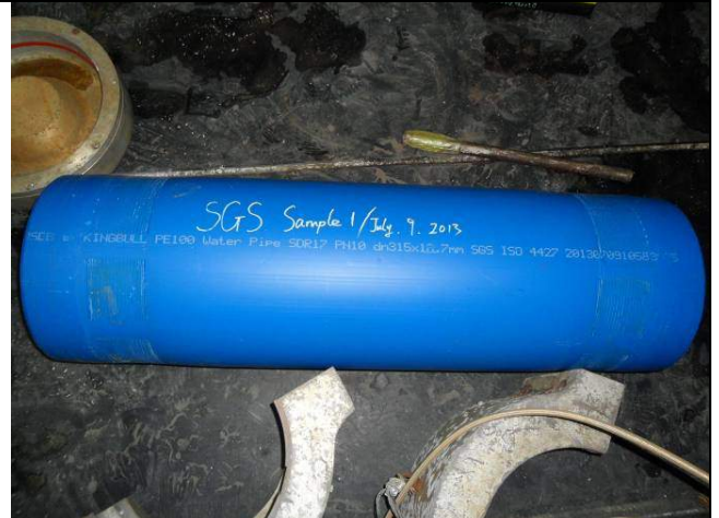
The PE pipe after hydrostatic test
