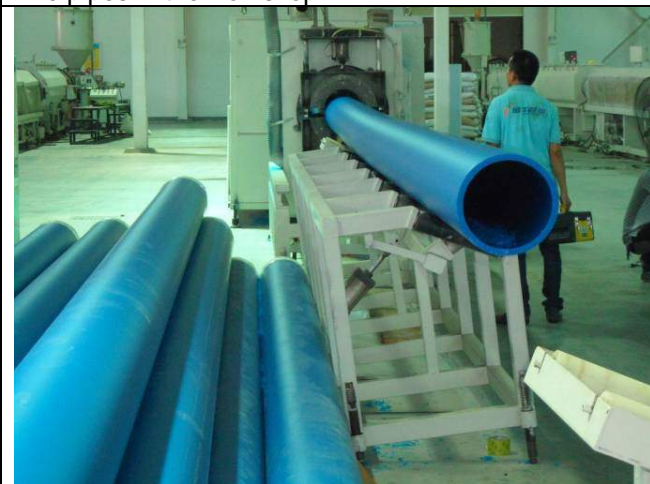
The pipe DN315 was in producing
