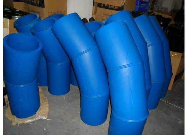
The PE fittings in the workshop
