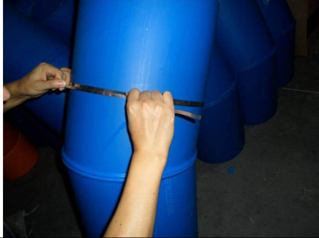
Mean outside diameter check of PE fitting
