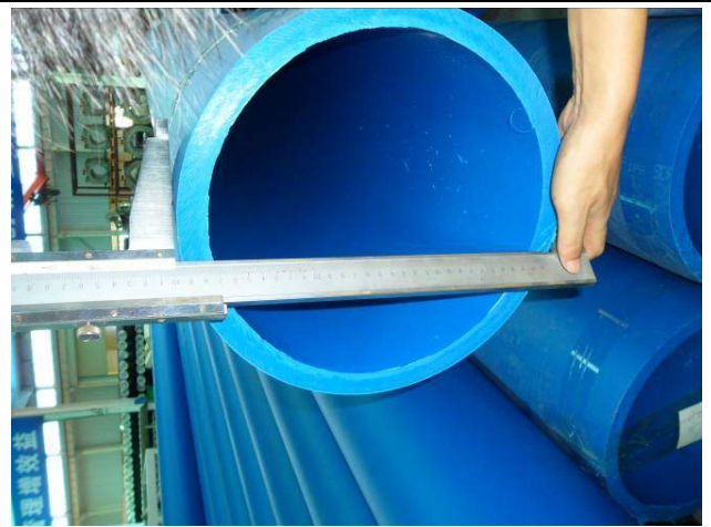
Out-of-roundness check of PE pipe
