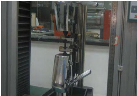
Elongation at break test
