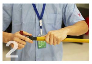
Round and bevel the endholes and make a no-less-than-2-minimeter incline.
