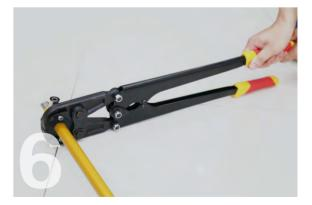
Press, make sure the moulds are clean and close completely when pressing.
