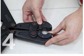
Choose the right size clamp by the mark on the moulds, matching the press fitting.
